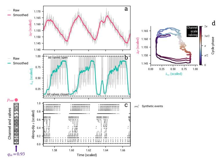
Figure 12. Cyclic variations of activity for  $q_{in}=0.93$ . (a) Pore pressure difference across the whole channel  $\Delta p$ , (b) channel bulk permeability  $k_{eq}$ , and (c) time-location chart of events. (d) Activity in  $(\Delta p, k_{eq})$  space, showing hysteretical cycles like those of a single valve. Valve distribution represented in Figure 2, valve parameters are listed in Table 2.
