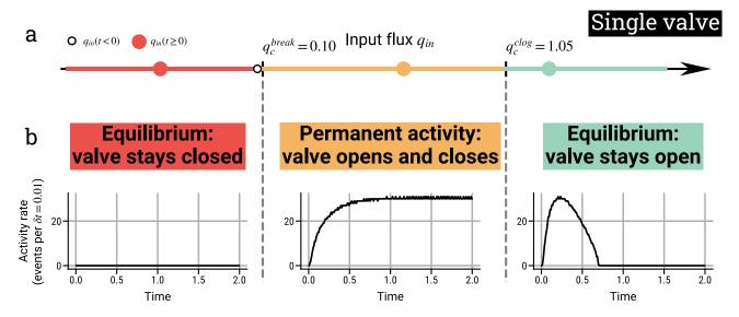
Figure 5. Influence of the input flux  $q_{in}$  on the activity of a single valve. (a) Three intervals of input flux  $q_{in}$  are delimited by two threshold values  $q_c^{clog}$  and  $q_c^{break}$ . (b) Examples of activity rate evolution in time (in black) for each regime. Activity rate is taken as the number of events per  $\delta t = 0.01$ , scaled unit. An event corresponds to the opening of a valve. Valve parameters are listed in Table 2.
