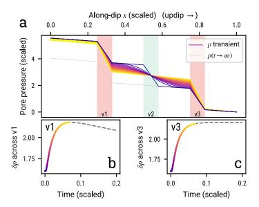
**Figure 6.** Interactions between three neighboring valves. (a) Transient evolution of pore pressure from an initial equilibrium profile with all valves closed toward a profile with valves v1 and v3 closed and valve v2 open. Panels (b) and (c): pore pressure difference evolution across valves v1 and v3.
